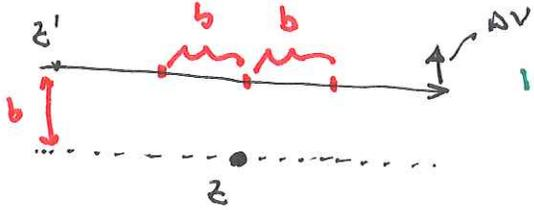
$$\text{Impulse} \approx F \Delta t = \frac{z'e e z}{4\pi\epsilon_0 b^2} \frac{2b}{v_0} = m \Delta v$$
