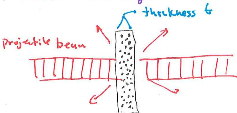
$$\begin{aligned} \text{fraction scattered} &= \sigma n_2 \\ \text{fraction scattered into } d\Omega &= \frac{d\sigma}{d\Omega} n_2 d\Omega \end{aligned}$$
