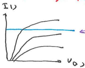
if we had a load line like this very small changes in  $V_G$  → big  $V_{DS}$  swings i.e. big gain
