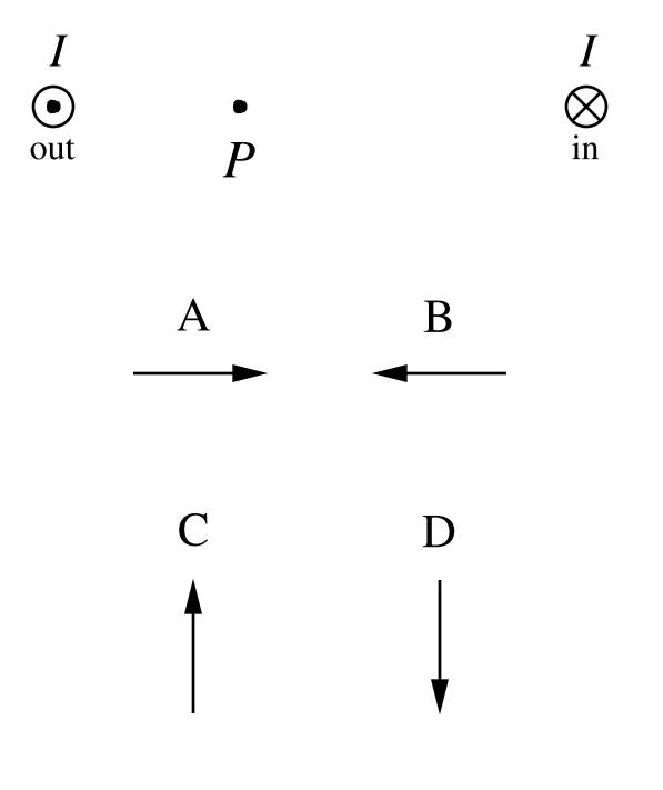
Wire 1 has a large current I flowing out of the page (•), as shown in the diagram. Wire 2 has the same current *I*, but flowing into the page  $(\otimes)$ . In what direction does the magnetic field point at position P?
