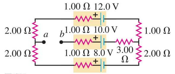
26.57 (a) Find the potential of point a with respect to point b in Fig. P26.57. (b) If points a and b are connected by a wire with negligible resistance, find the current in the 12.0 V battery.
