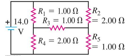
26.62 (a) Find the current through the battery and each resistor in the circuit shown in Fig. P26.62.
