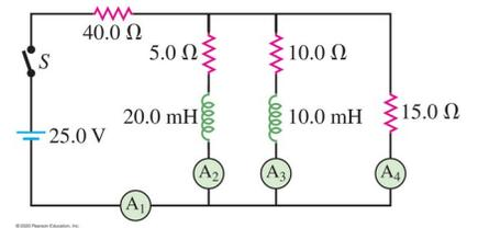
30.58 CP In the circuit shown in Fig. P30.58, find the reading in each ammeter and voltmeter (a) just after switch S is closed and (b) after S has been closed a very long time.
