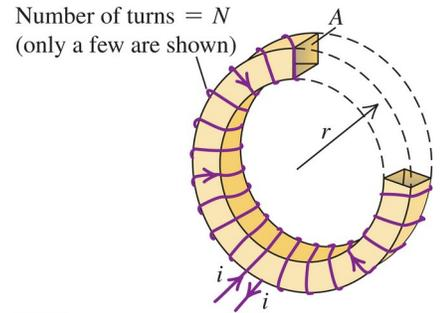
30.6 A toroidal solenoid has 500 turns, cross-sectional area  $6.25 \text{ cm}^2$ , and mean radius  $4.00 \text{ cm}$ . (a) Calculate the coil's self-inductance. (b) If the current decreases uniformly from  $5.00 \text{ A}$  to  $2.00 \text{ A}$  in  $3.00 \text{ ms}$ , calculate the self-induced emf in the coil. (c) The current is directed from terminal a of the coil to terminal b. Is the direction of the induced emf from a to b or from b to a?
