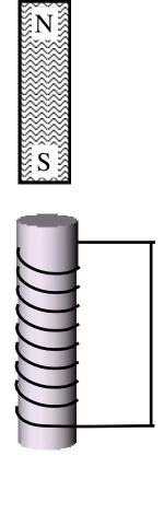
The south pole of a bar magnet has been sitting near the end of a solenoid. The bar magnet is now moved vertically towards the solenoid. Which way will the current flow in the straight section?
