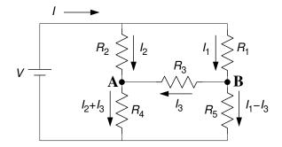
Applying Kirchhoff's laws, write down the linear equations needed to determine the currents  $I_1, \ldots, I_5$ , where V and  $R_1, \ldots, R_5$  are known constants. If you solve these equations (solving is not required) you'd find  $I_3 = 0$  if  $R_1/R_5 = R_2/R_4$ .
