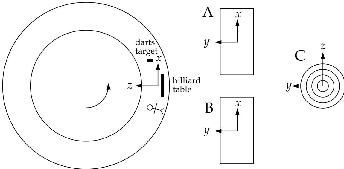
4. Imagine your experience in a ‘big wheel’ space station whose living apace is a torus with radius  $R = 10$  m and is rotated so the centrifugal force is equivalent to the force of gravity on the surface of the Earth:  $mg$ . Your  $x$  axis aligned with the wheel’s circumference and points in the direction of the wheel’s tangential velocity, your  $z$  axis points toward the center of the wheel (i.e., in the apparent ‘up’ direction) and your  $y$  axis points to your left.
