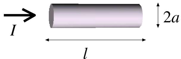
A resistor consists of a long cylinder of carbon (radius  $a$ , length  $\ell$ ) and carries a current  $I$ . If a bit of the carbon cylinder is cut off (reducing the length  $\ell$ , but not changing the current  $I$ ) report how the below quantities would change.
