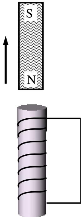
The north pole of a bar magnet is moving away from the solenoid
