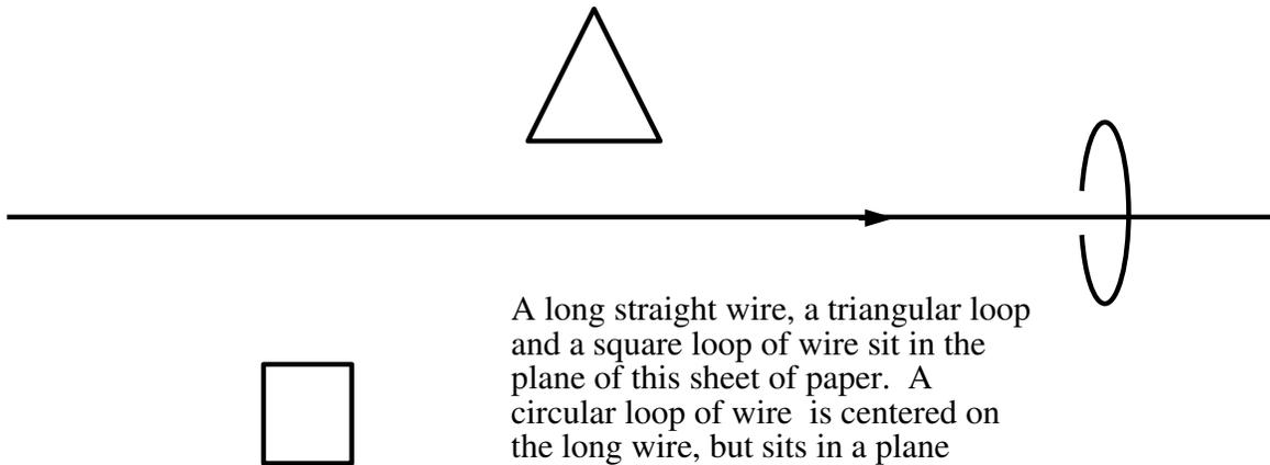
A long straight wire, a triangular loop and a square loop of wire sit in the plane of this sheet of paper. A circular loop of wire is centered on the long wire, but sits in a plane perpendicular to the long wire. For several minutes there has been a current flowing to the right; that current is now decreasing.
