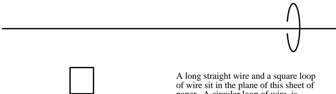
A long straight wire and a square loop of wire sit in the plane of this sheet of paper. A circular loop of wire is centered on the long wire, but sits in a plane perpendicular to this sheet of paper. For several minutes there has been no current flowing in any wire. A battery (not shown) is connected and a current starts to flow to the left through the long straight wire.
