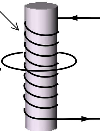
For several minutes no current has been flowing through the primary circuit. A current now starts and increases in the direction indicated. Place an arrow on the front surface of the secondary circuit showing the direction of any resulting current induced in the secondary circuit
